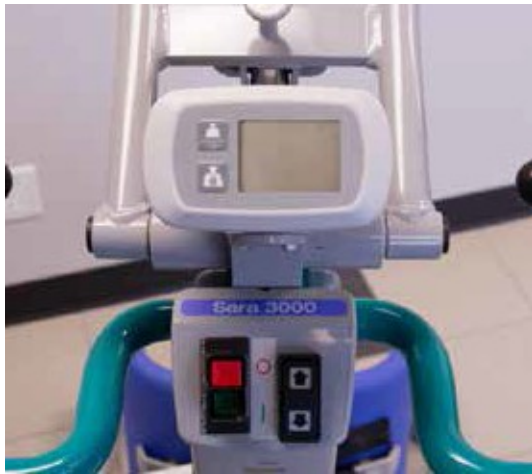
The optional integrated scale saves time by weighing the resident during a transfer.
